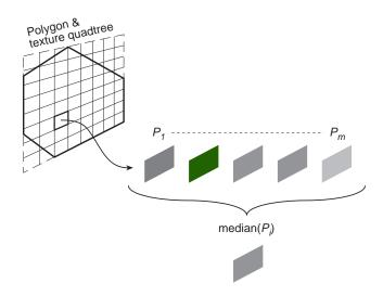
Figure 5: Pixel stack from one quadtree node and occlusion detection in principle.
