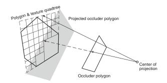
Figure 4: The influence of occluder polygons to the quadtree structure.
