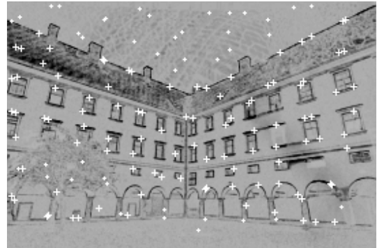
(c) Visualization of our accuracy measure; Crosses indicate corresponding points used for the calculation of the relative orientation.
