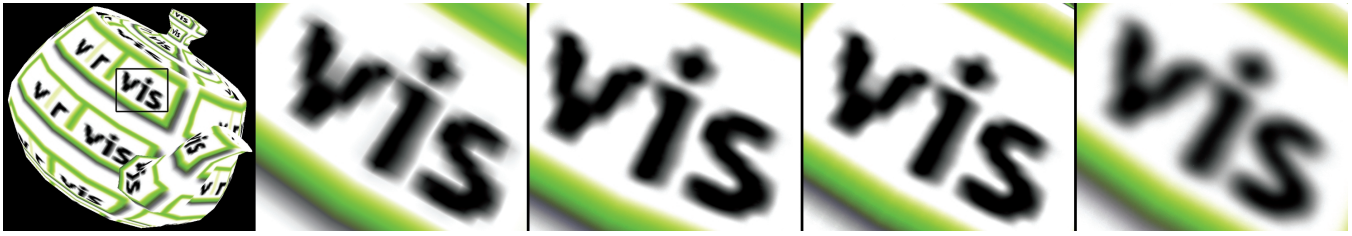
Figure 3: Filtering a 64 \times 64 texture mapped several times onto a geometric object; from left to right: bi-linear interpolation, Catmull-Rom spline, Kaiser-windowed sinc, cubic B-spline. The corresponding frame rates are shown in table 5.
