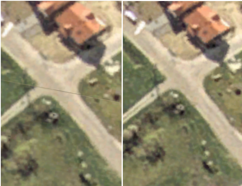
Figure 2: a) Texture split with seams on the left. b) Corrected textures on the right
