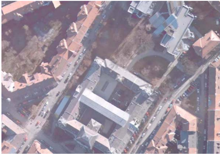
Figure 4: 3D view of the textured DSM with the projection mode set to orthonormal projection and a vertical viewing direction. The facade surfaces are not visible, as expected from a ‘true’ orthophoto.
