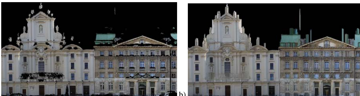
Figure 8: a) Orthonormal projection of the dense point cloud shown in Figure 7. b) Areas with no visibility to any input image are filled with color information from surrounding regions.
