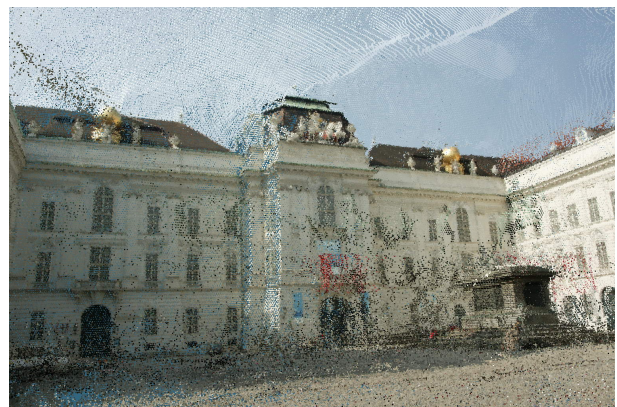
Figure 2: Dense point cloud of one side of the Josefsplatz in Vienna. As a consequence of the outliers (sky, ground) in the created reconstruction a pre-segmentation of the scene in meaningful units like facades and roofs is necessary.
