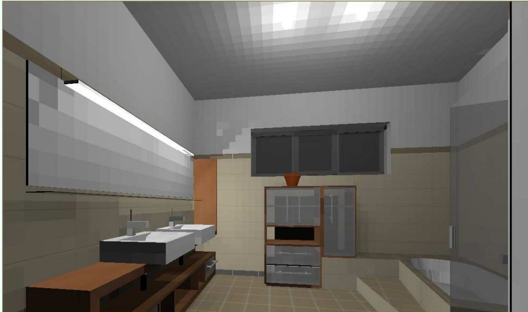
Figure 2: Hardware accelerated combination (No bilinear filter as GeforceFX does not support this for float-textures), combination every frame - 25fps
