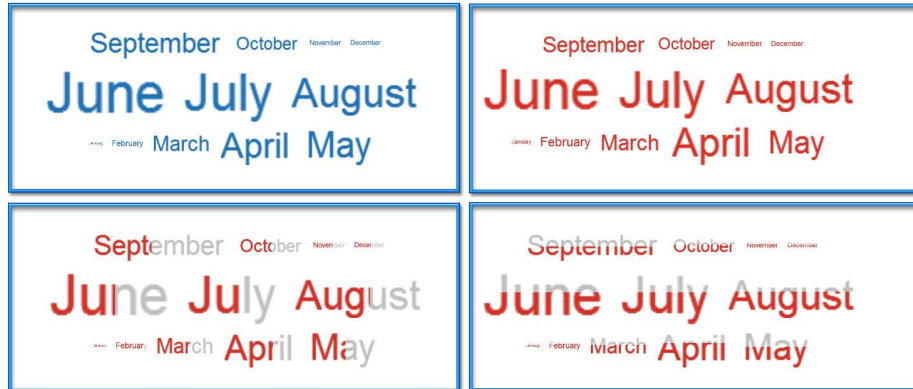
Fig. 3. The tag cloud view integrated in the CMV system. The top left tag cloud view shows months as contained in our data set. The user selected only the interdiction region (in a histogram view not showed here) and the selection is shown with context in the lower row (horizontal and vertical), and without the context in the top right tag cloud view.
