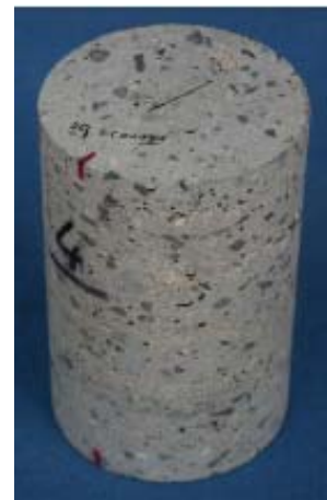
Fig. 4: One of the drill core samples of a tunnel lining used for the investigations.
