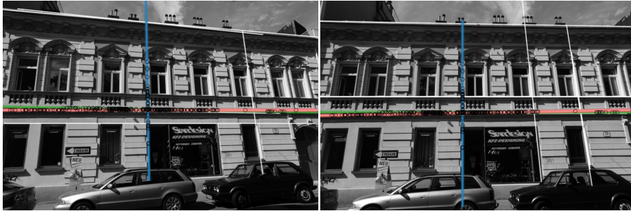
Fig. 5. Facade scene: 365 point correspondences in four lines. Matching lines are displayed with the same color, unmatched lines are shown in white. The final point correspondences are visualized as black rings. Note that some lines are collapsed because they are located very near to each other.
