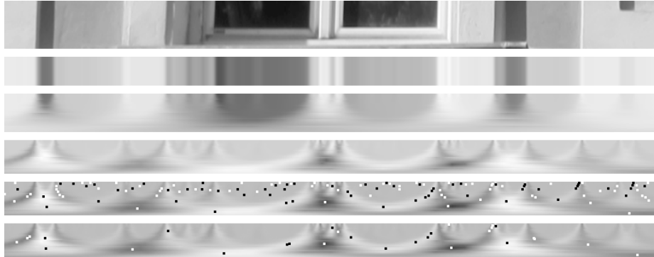
Fig. 2. From top to bottom: sampled rectangle next to a line segment, collapsed profile, Gaussian scale space with 6 octaves and 5 scales per octave, DoG scale space, extrema (white and black dots) in DoG scale space, accepted feature points with refined positions in DoG scale space.
