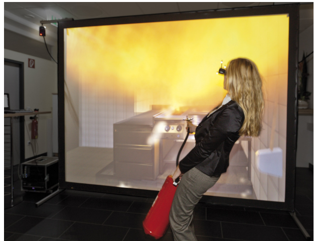
Figure 2: User engagement with the aid of a stereoscopic display. The trainee is able to interact in a 3D space by shutter glasses and a stereoscopic display. Image courtesy of Maschek [7]
