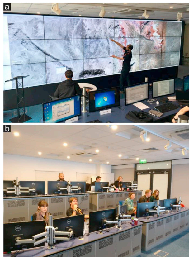
Fig. 5. MOC setup. a) The large video wall. The desktop view of one workstation could be stretched over the whole wall, as here, or several workstation desktops could be split across the screen ‘on the fly’. b) The tiered workstations for the SWT stations. Image credit: Andrew Griffiths.
