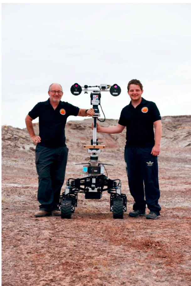
Fig. 1. The MURFI 2016 rover: a ‘Q14’ platform with PanCam emulator ‘AUPE’ (Harris et al., 2015) attached. The large “eyes” contain the filter wheels for the PanCam emulator. Field team for scale. Image credit: Mike Curtis-Rouse.
