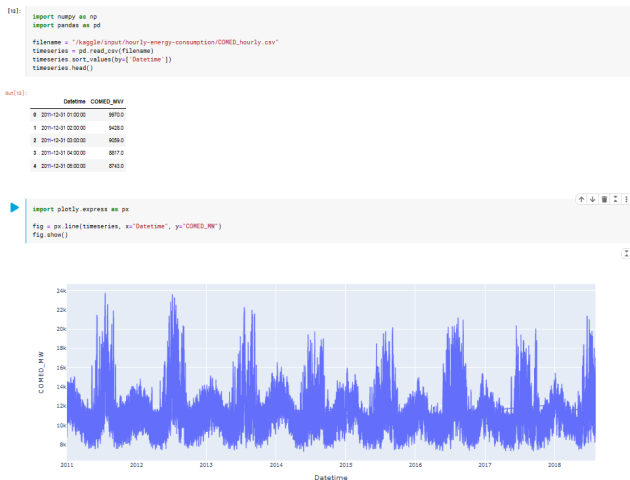
Figure 1: Notebook application. Here two cells in a Kaggle notebook are shown, containing Python code to load a timeseries dataset and an inline visualization to plot the data.
