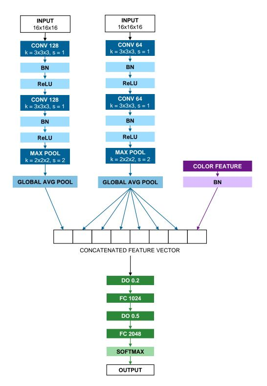
Figure B.2: Architecture of the network using middle grid size.
