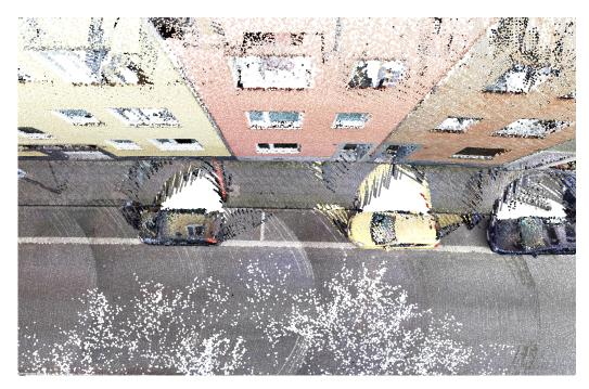
Figure 6.21: The LiDAR point cloud of the street named "Kleiner Griechenmarkt" from above.
