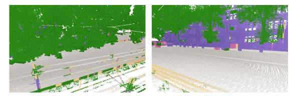
Figure 6.5: The result of the semantic segmentation of the network using big grid size and six classes of the street named "An der Schanz".
