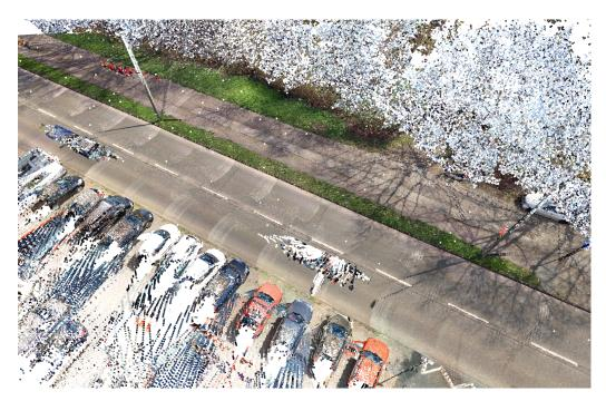
Figure 6.16: The LiDAR point cloud of the street named "Äußere Kanalstraße".
