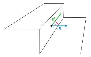
Figure 4.3: Perpendicularity feature, where the angle between the point normal n and the direction of the road d is computed.
