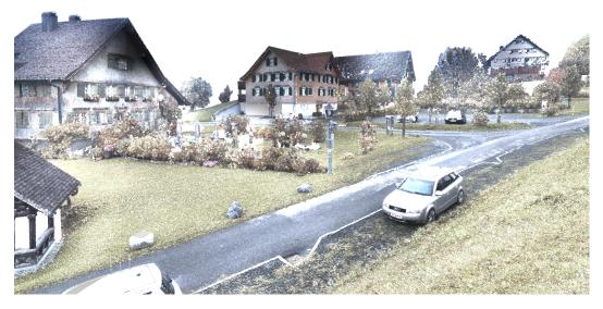
Figure 3.5: A point cloud of the Semantic3d dataset, captured with a laser scanner in a rural area.
