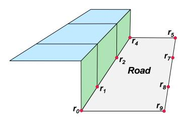
Figure 4.10: The final polygons of a curb section from three curb as well as sidewalk segments and the road polygon, which is constituted by the vertices  $r_i$ .
