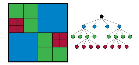
Figure 3.1: 2D visualization of an octree.
