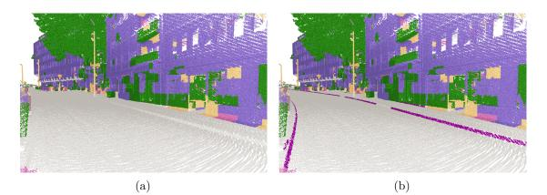
Figure 6.13: (a) The result of the semantic segmentation with the network using big grid size and six classes. (b) The result of the geometrically calculated curb feature points of the street named "Augustinerstraße".
