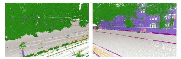
Figure 6.6: Detected curb points coloured magenta of the geometric feature calculation of the street named "An der Schanz".
