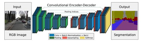
Figure 2.6: Semantic segmentation network architecture with encoder-decoder structure. (Source: [BKC17])
