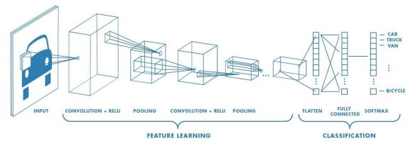
Figure 3.7: Exemplary structure of a CNN illustrating its two-stage structure with the *feature learning* and *classification blocks*. (Source: [Sah])
