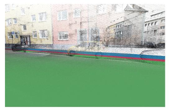
Figure 6.22: The final reconstructed geometry of the street, curb and sidewalk of the street named "Kleiner Griechenmarkt".
