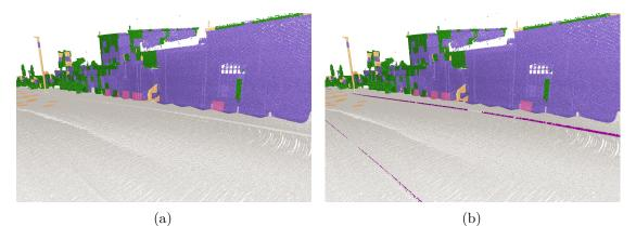
Figure 6.10: (a) The result of the semantic segmentation with the network using big grid size and six classes. (b) The result of the geometrically calculated curb feature points of the street named "Auenweg".
