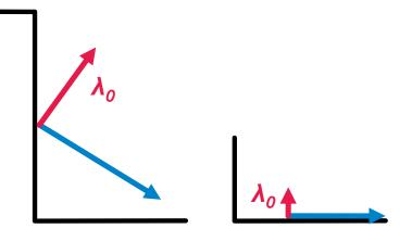
Figure 4.2: Result of an eigenvalue decomposition, once from a curb point (left) and once from a street-point (right) in 2D. The eigenvalue  $\lambda_0$  from a curb point is larger than the eigenvalue  $\lambda_0$  from a street-point.
