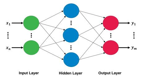
Figure 2.3: A visualization of a feedforward neural network, also known as multilayer perceptron (MLP).
