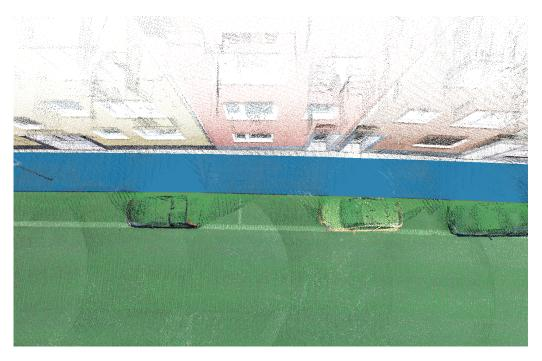
Figure 6.23: The final reconstructed geometry of the street, curb and sidewalk of the street named "Kleiner Griechenmarkt" from above.
