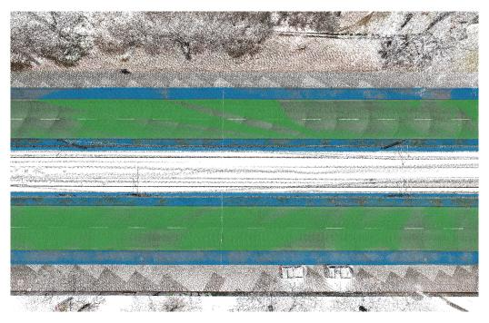
Figure 6.8: Top view of the reconstructed geometry of the street named "An der Schanz" of both lanes.
