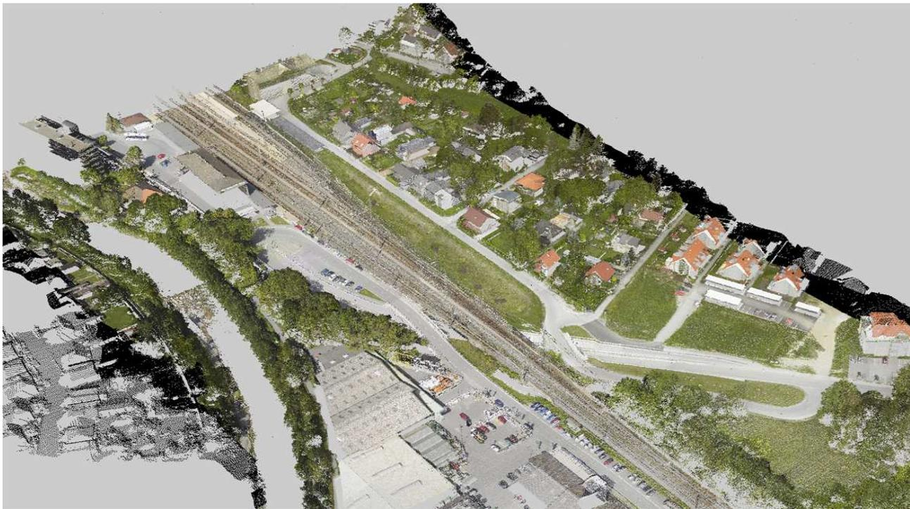
Figure 3: Laser scan data colored by orthophotography.
