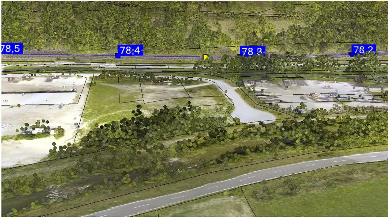
Figure 5: Close-up view. In addition to the terrain and vegetation data, GIS meta-information depicts property boundaries and railway chainage labels (in kilometers).
