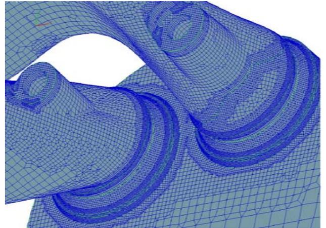
Figure 1: A close-up view of two intake ports in a same CFD simulation grid. The mesh contains multiple, adaptive resolution levels of unstructured grid cells.
