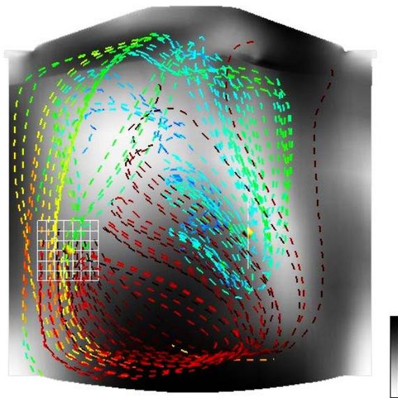
Figure 4: The visualization of tumble motion using animated, dashed streamlines. Two seeding planes are used: one seeding color mapped streamlines, the other emanating red streamlines. A gray-scale mapped slice serves as context information.
