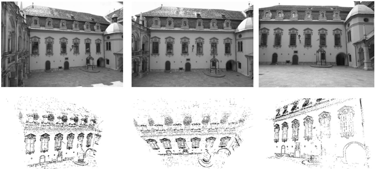
Figure 10: Top row: Three of the five images used of the courtyard scene (image size =  $2160 \times 1440$ ). Bottom row: Three views of resulting 3D point cloud.
