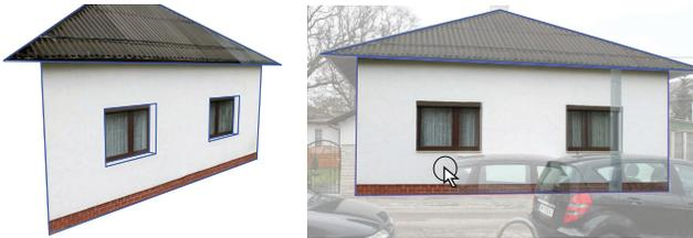
**Figure 6:** *Left: By defining hierarchical relations, holes and side faces are automatically extracted. Right: Interactive removal of occluding objects from the texture by overlaying the photo semi-transparently using the shot view.*
