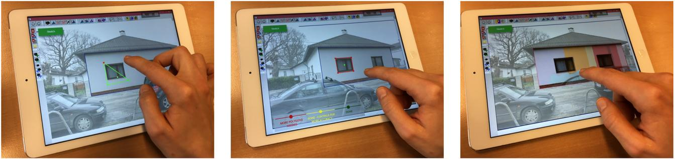
**Figure 8:** Evaluation of our proposed system on a touch-based device. Left: Coarse sketching of the polygon in the initial view. Middle: The polygon has been snapped to image edges and been reprojected to a neighboring image in the multi view sketching mode. The visual guidance feedback indicates that enough views have been used. Right: Interactive brushing.
