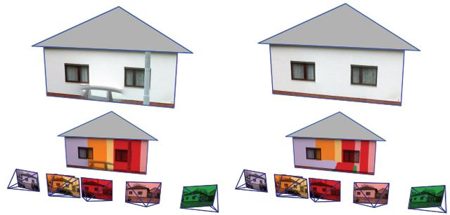
**Figure 7:** *Top left: The initial texture containing occluders. Bottom Left: The associated shots, visualized using a false color mask. Top right: The cleaned texture after interactive brushing. Bottom right: The correspondingly modified mask.*
