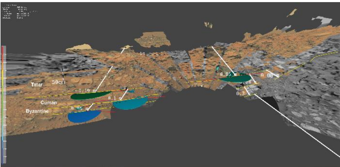
Figure 6: Geologic annotation/interpretation of MER-A Sol 748-751 (Gibson Formation) Pancam PRoViP stereo-to-OPC processing result. This was used as data collected during Sol 49 of Sim#2, and was used to measure the true thickness of the units (thick white lines), and the dip and strike of the key boundaries and internal layers (disks and arrows coloured by dip magnitude, the red lines represent the strike direction). Credits: NASA/JPL-Caltech/MSSS/ASU
