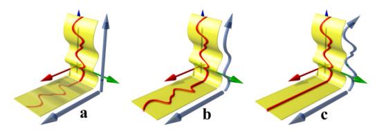
Figure 2: Different CPR generation methods: a) Projected CPR, b) Stretched CPR, c) Straightened CPR
