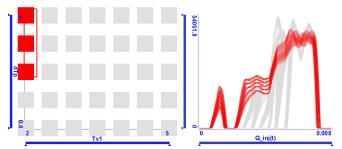
Fig. 14. If the injector valve is opened very early than the injection rate quickly increases to the "boot" level. It reaches its maximum when the mixture is ignited in the combustion chamber.
