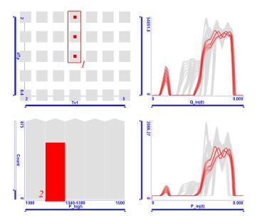
Fig. 13. Top left: brush 1 selects control parameters for ramp shaped main injections. Bottom left: brush 2 is probed in the histogram of the high pressure on injector inlet using the AND operation. Top right: injection rate function graphs of the brushed items. Bottom right: injection pressure function graphs of the brushed items. By dragging brush 2 and studying the linked function graph view we observe that injection rate function graphs have similar shapes but different maxima.
