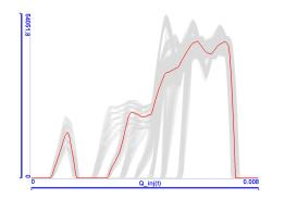
Fig. 7. A typical shape of the fuel injection rate function graph is highlighted in red. There is a short pilot injection first, followed by the main injection. The function graphs resulting from other combinations of control parameters are gray.
