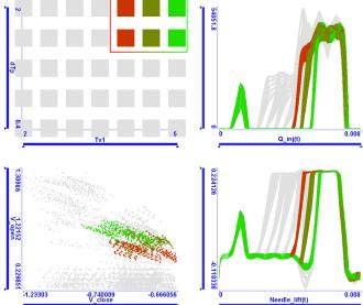
Fig. 12. Required needle movement characteristics for square shaped main injections. Top left: control parameters that produce square shaped injections are brushed. Top right: red to green gradient shows that earlier valve opening times cause deviation from the ideal square shape. Bottom left: needle opening and closing velocities must be fairly high for this shape. Bottom right: the shape of the needle lift function graph is closely correlated to that of the injection rate function graph.
