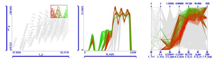
Fig. 15. We investigate the conditions when fuel is injected deep in the combustion chamber and with high power. The corresponding items are brushed in the scatterplot diagram. The linked injection rate function graphs show that this requires boot shaped main injections. The desired needle opening and closing velocities are highlighted in the parallel coordinate view.
