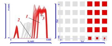
Fig. 11. Ranges of control parameters that produce square shaped injections. First the user attempted to select square shaped graphs with brush 1. This brush selects several not square shaped graphs, too. These are removed by subtracting graphs that intersect brush 2. Brush 3 removes graphs that drop under a certain threshold in the main injection part. This property is a result of vibrations in the fuel line, which are to be avoided.
