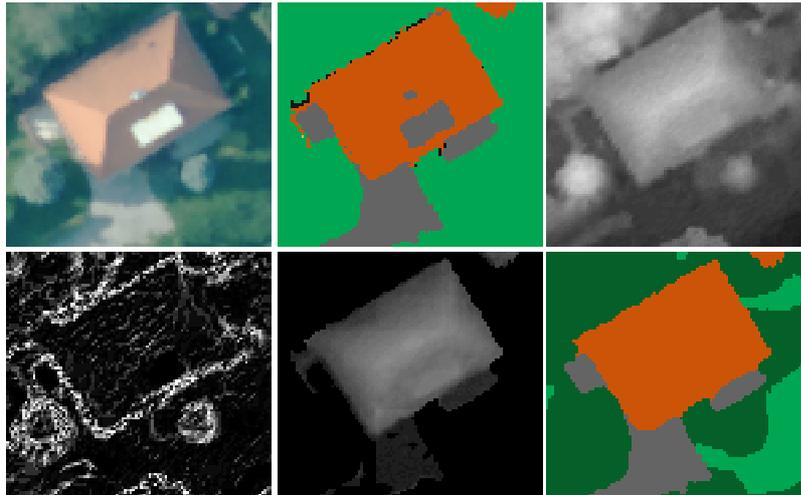
Figure 5: Different stages within our modeling workflow. Top row: one input image (left); initial LUC (middle); height image produced by dense matching (right). Bottom row: height gradients (left); fusion of LUC and height image; refined LUC (right).
