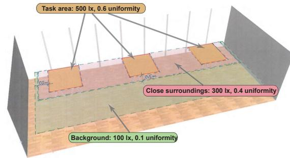
Fig. 2. Conceptual sketch made by a lighting design expert, defining the location of the measurement surfaces and their target values in the office scene according to industry standards [8].
