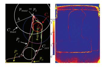
Figure 2: From left to right: a) Hand detection output and palm detection diagram; b) Standard deviation of background measurements over 100 frames.
