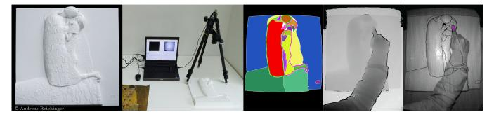
Figure 1: From left to right: a) Tactile relief interpretation of Gustav Klimt's "Der Kuss" (The Kiss, 1908/09); b) Test setup; c) Label image, warped to camera space. Outlines indicate merged base labels; d) Depth image; e) Infrared image with superimposed label borders and touched label (purple). © Andreas Reichinger
