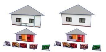
Figure 7: Top left: The initial texture containing occluders. Bottom Left: The associated shots, visualized using a false color mask. Top right: The cleaned texture after interactive brushing. Bottom right: The correspondingly modified mask.
