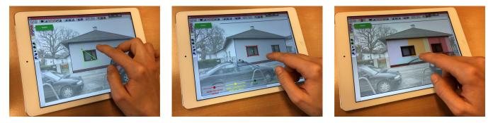
**Figure 8:** Evaluation of our proposed system on a touch-based device. Left: Coarse sketching of the polygon in the initial view. Middle: The polygon has been snapped to image edges and been reprojected to a neighboring image in the multi view sketching mode. The visual guidance feedback indicates that enough views have been used. Right: Interactive brushing.
