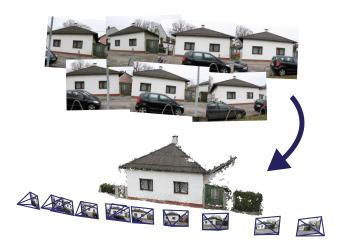
**Figure 2:** *Photogrammetric Network (bottom), consisting of a 3D point cloud and photos (top), for which their relative positions and orientations have been computed. We refer to them as shots.*
