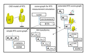
**Fig. 13** Exemplary scene graphs for for RTS simulators, including following nodes: Scene node (reference frame), environment node (measurement targets), RTS (device model). Simple scene graph: no visualization of the kinematics of the individual RTS components. Extended scene graph: DH parameters can be applied to the individual RTS components
