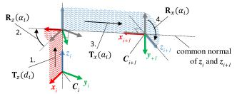
**Fig. 2** Relative pose  $\mathbf{M}_{i,i+1}$  of frame i + 1 with respect to frame *i* as defined by the DH convention
