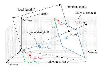
Fig. 1 Simplified kinematics model used in [21]
