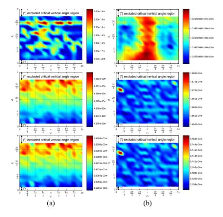
**Fig. 11** Modeling error distribution with respect to the angle control parameter space, using Eq. 92 for each control point { $\varphi_i$ ,  $\theta_i$ }. **a** Optimized with reduced parameter space. **b** Optimized with full parameter space. End effector error (method B), encoded as color: EDM (top row), camera (middle row), compound (bottom row)
