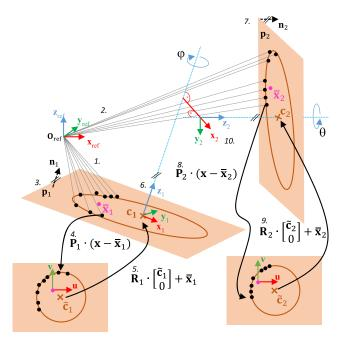
**Fig. 4** Circular feature extraction. The algorithm steps are labeled in ascending order: 1,2: measure points; 3,7: fit plane; 4,8: project to 2D; 5,9: fit circle and transform result to 3D; 6,10: define frames
