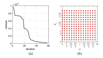
Fig. 9 a Residual evolution of SQP optimization. b Angle control parameter space for cross-validation
