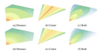
Figure 2: Point density reduction by distance to camera, distance to the center of the screen, and both. Top-row: Filtering based on the level of a point inside the hierarchy, with sudden drops in density. Bottom-row: Continuous results with dither-like patterns after adding a random value between 0 and 1 to the level of each point. Colors represent the level attribute of a point.
