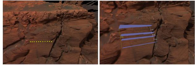
Figure 6: Picking points on a sedimentary line (left) to create a true-layer-thickness stack (right).
