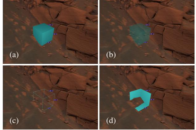
Figure 3: Four draw modes for scale-boxes: (a) solid, (b) transparent, (c) wirebox, (d) frontface culling.
