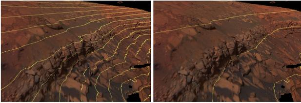
Figure 7: Adjustable spacing and offset for contour-lines. Left: 0.5 m spacing, right: 2 m spacing.
