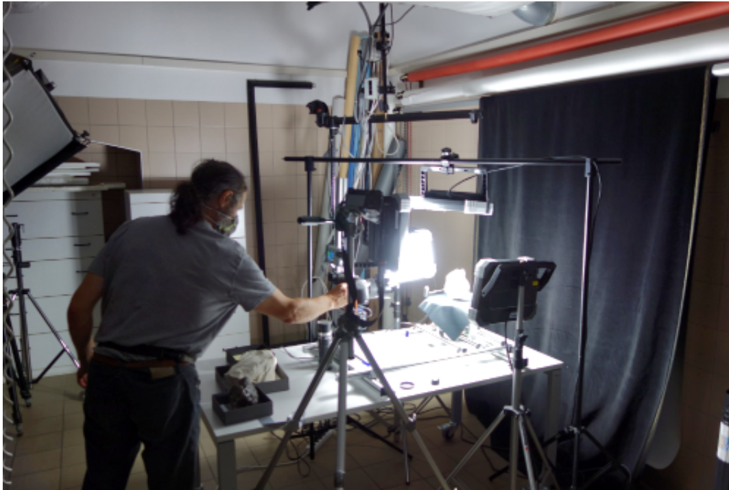
Figure 2: Capturing shatter cones with homogeneous lighting.
