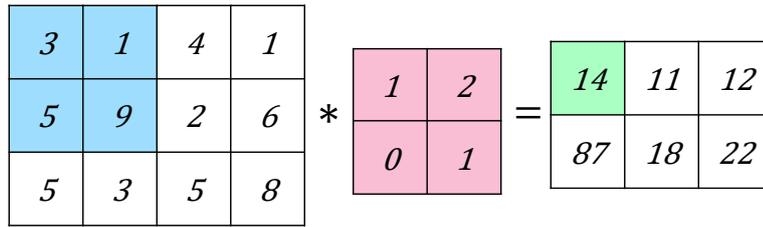
Figure 2.4: An example of a convolution operation. Such an operation  $conv = m * k$  consists of an image matrix  $m$  and a kernel  $k$ . The kernel shifts like a sliding window over the image matrix and computes new image values by multiplying and adding according values. The position of the sliding window is visualized in blue, the kernel in pink and the resulting value in green, which is obtained as follows:  $3 * 1 + 1 * 2 + 5 * 0 + 9 * 1 = 14$ .
