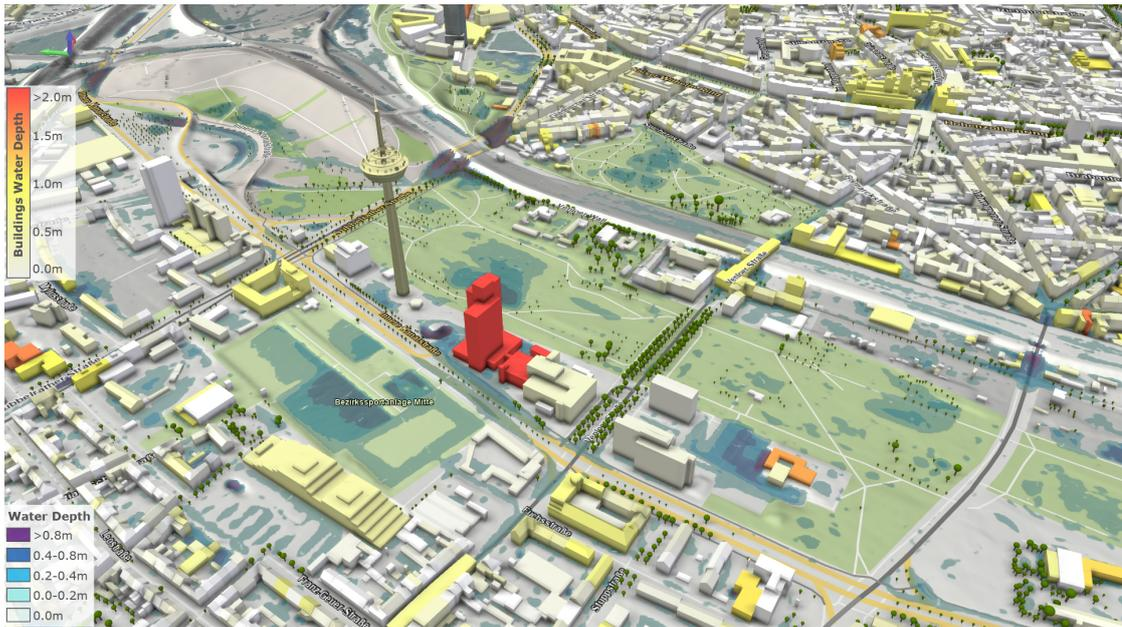
Figure 1.1: Screenshot of the Visdom flood simulation software. (Source: [Vis])
