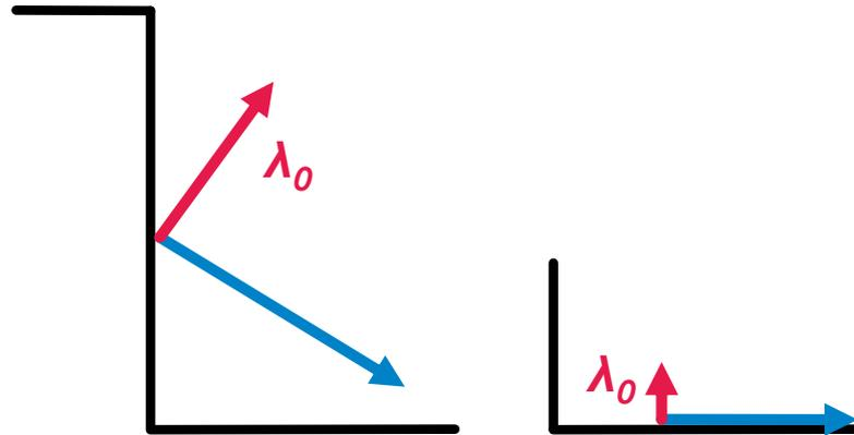
Figure 4.2: Result of an eigenvalue decomposition, once from a curb point (left) and once from a street-point (right) in 2D. The eigenvalue  $\lambda_0$  from a curb point is larger than the eigenvalue  $\lambda_0$  from a street-point.
