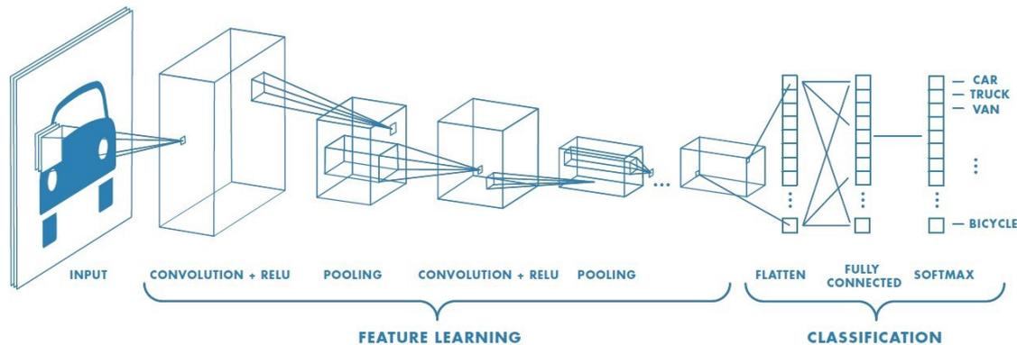
Figure 3.7: Exemplary structure of a CNN illustrating its two-stage structure with the *feature learning* and *classification blocks*. (Source: [Sah])
