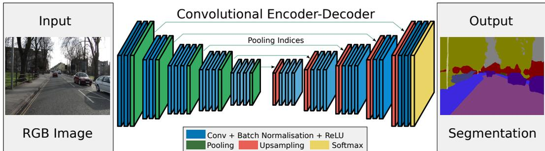
Figure 2.6: Semantic segmentation network architecture with encoder-decoder structure. (Source: [BKC17])
