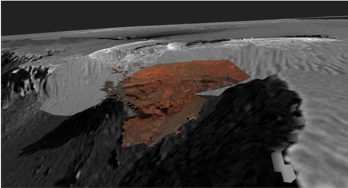
Figure 6.2: The Victoria Crater scene has in total 2.3 GB. LOD 0 has 1.3 GB and 17.7 million triangles. The colored mesh shows data of a higher-quality layer rendered with priority rendering.
