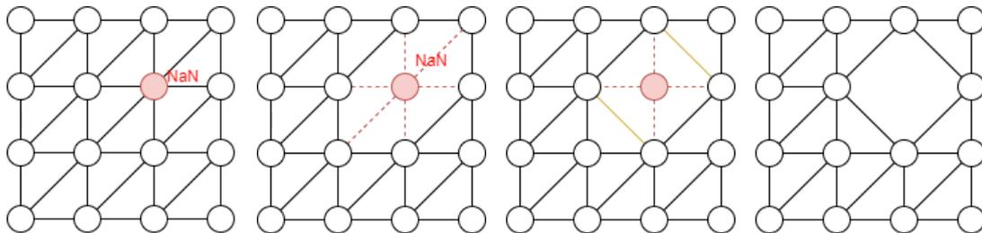
(a) *NaN* value detected. (b) *NaN* value removed (c) Re-Triangulation (d) Resulting hole.
