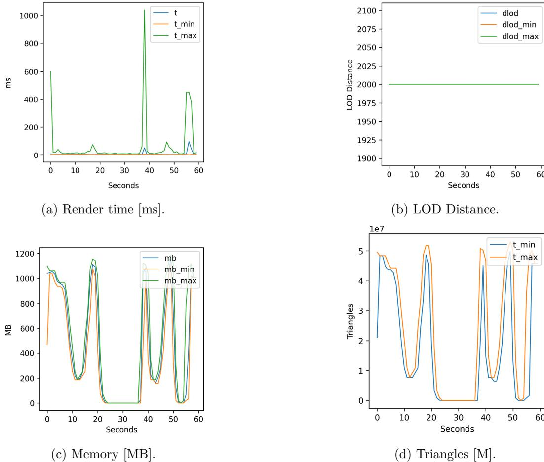
Figure 6.6: (a) The average render time is well below 50 ms. (b) The reactive target frame-rate scheduler does not react to the single spike around the 40 s mark, caused by loading almost all LOD nodes back in when zooming out. (c) The sharp drop in memory and triangle counts (d) close to 0 MB used of memory clearly show that Visionary is too aggressively releasing currently not required nodes.
