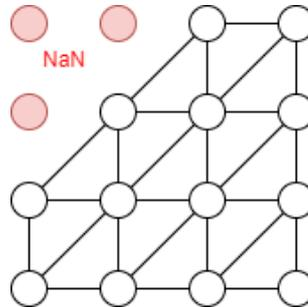
Figure 5.12: *NaN* values are used to mark the border of a non-rectangular patch.
