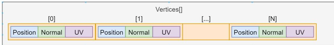
(b) Position, normal and texture coordinate are combined per vertex and stored as an array of *VertexData*. This memory layout is used during rendering and allows to copy the read data directly into the target GPU buffer.
