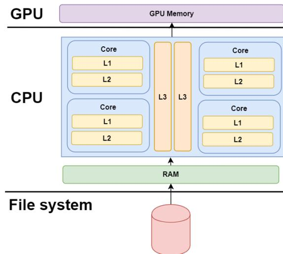
Figure 5.15: Modern CPUs and GPUs have sophisticated multi-layer cache architectures. Both have dedicated caches for specific operations. The CPU cache architecture shown is a schematic representation of the Zen 2 cache architecture and shows a per core L1 and L2 cache model with a shared L3 cache [Naf+21].
