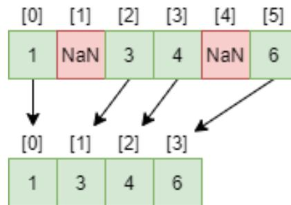
Figure 5.14: Discarding invalid NaN values leaves array indices [1] and [4] unused. By shifting all data left, the arrays become compact again. No unused indices remain. All aligned arrays have to be shifted accordingly.
