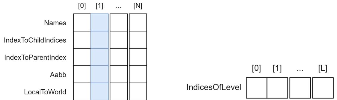
(a) Data per node is stored in aligned arrays. The data of *node 1* (blue) is stored at *index 1* of each aligned array.
