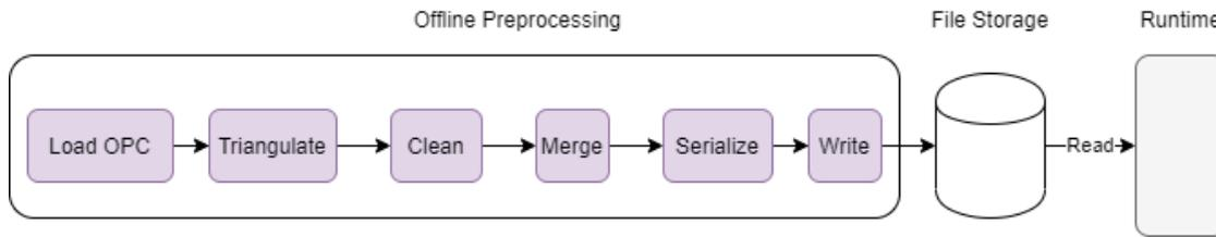
Figure 5.10: The pre-processing stages in order. Pre-processing ends with writing the serialized files back to the filesystem.
