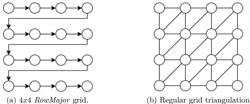
Figure 5.11: RowMajor linearized arrays store the data row by row. Given the width and height of the 2D grid, a regular grid triangulation is possible.
