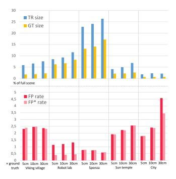
Fig. 15. Average PVS size tightness for various scenes and viewcell sizes  $|\Delta|$ . In the top chart, "TR size" and "GT size" indicate the percentage of the full scene placed in the PVS of the trim region method and the ground truth, respectively. In the bottom chart, "FP rate" and "FP\* rate" indicate the false positive rate (as a multiple of the ground truth) without and with suppression of unreliable primitives, respectively.
