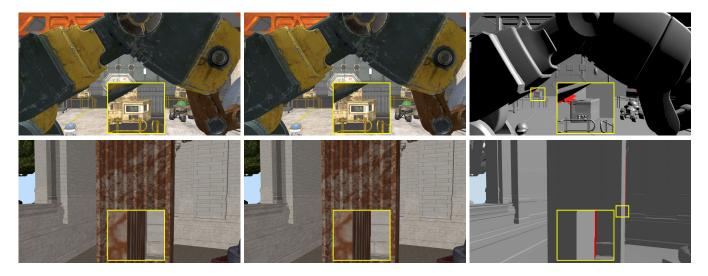
Fig. 17. Challenging situations in Robot lab (top row, 210 false negative pixels) and Sun temple (bottom row, 344 false negative pixels). In each row, the left column shows the full scene; the middle column shows the PVS computed by TR, and the right hand side highlights false negative pixels in red. The differences to the full scene are not immediately apparent in the PVS rendering.
