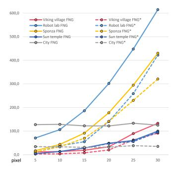
Fig. 16. Average false negative pixel count per frame for all possible views. FNG (solid lines) show results with unreliable triangles;  $FNG^*$  (dashed lines) shows results without unreliable triangles. When applying the cut-off suggested by Wonka et al. [2006] of roughly 100 pixels, a viewcell size of 15-20 cm can usually be supported without any noticeable errors.
