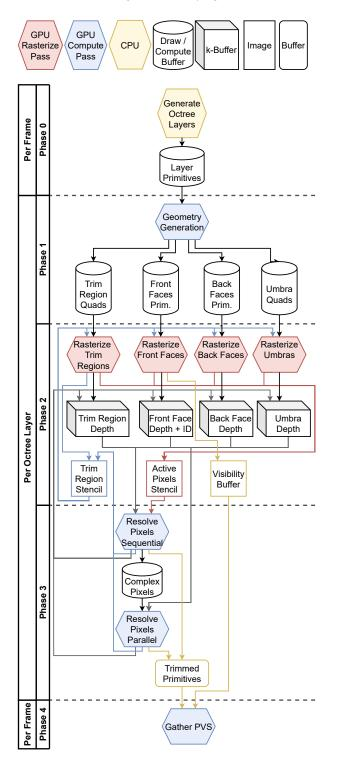
Fig. 8. The trim region algorithm commences in five phases: P1 determines the octree layers on the GPU. P1 generates the draw buffers for each layer, and P2 renders them. P3 resolves the resulting trim sequences. P4 gathers the results into the final PVS.
