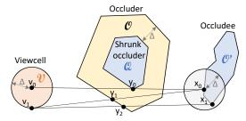
Fig. 3. The erosion theorem states that determining from-point visibility with respect to a shrunk occluder Q is equivalent to from-region visibility of the original occluder O. Any ray emitted from within a viewcell  $\mathcal{V}$  formed around  $\mathbf{v}_0$  cannot observe an occludee O', if O' is blocked by Q from  $\mathbf{v}_0$ . Even the extremal point  $\mathbf{v}_1$  in  $\mathcal{V}$  cannot see the extremal point  $\mathbf{x}_1$  of O'.
