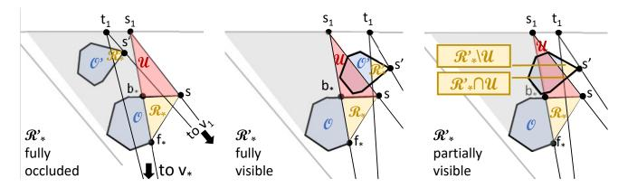
Fig. 5. (left) An occluder O spawns a trim region at silhouette s. After removing the trim region, the remaining parts of O still occlude portions in the back (gray and red areas). A trim region (yellow) of the occludee O' at s' is entirely occluded by O and does not contribute to the PVS. (middle) No intersection with the umbra produces a fully disoccluded occludee, while an intersection (right) produces a partly disoccluded occludee.
