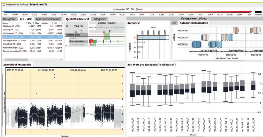
Analysis of the deviation of a quality indicator from the setpoint in different views, e.g. over time, averaged per order, distribution per batch etc.
